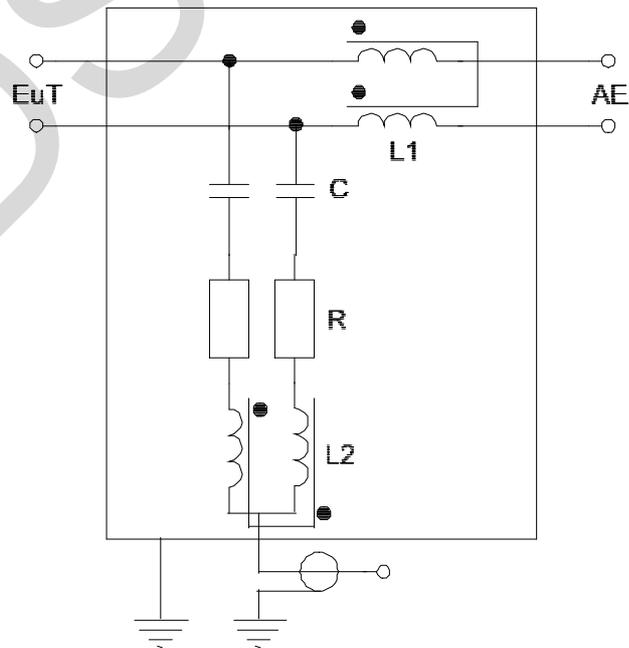
$$L1 = L2 = 2 \times 38 \text{ mH}, C = 0.47 \mu\text{F}, R = 200 \Omega$$
